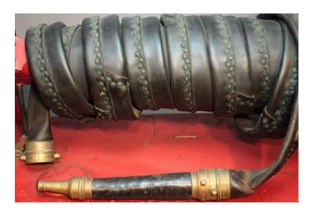
Metal-riveted leather hose was heavy, however. Fifty-foot lengths weighed about 85 pounds, and excluding couplings. Nor was leather hose very flexible. It became stiff with use, and difficult to roll or fold. Thus drums (or reels) were developed for transporting the hose. Short (single?) could be wound on a reel on the hand-engine itself. Longer lengths could be wound on reels mounted on a two- or four-wheel wagon.
