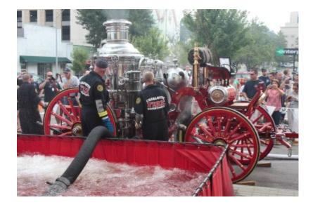
After heating the boiler for about 30 minutes, the Engineer and his crew were ready to flow water. The pump was engaged, the pistons started
