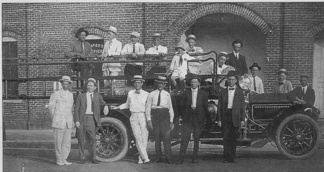
Members of the Oxford Fire Company stand with the 12-cylinder pumper truck the town purchased in 1925. The vehicle needed three men to turn it when it was moving because it had no power steering.
