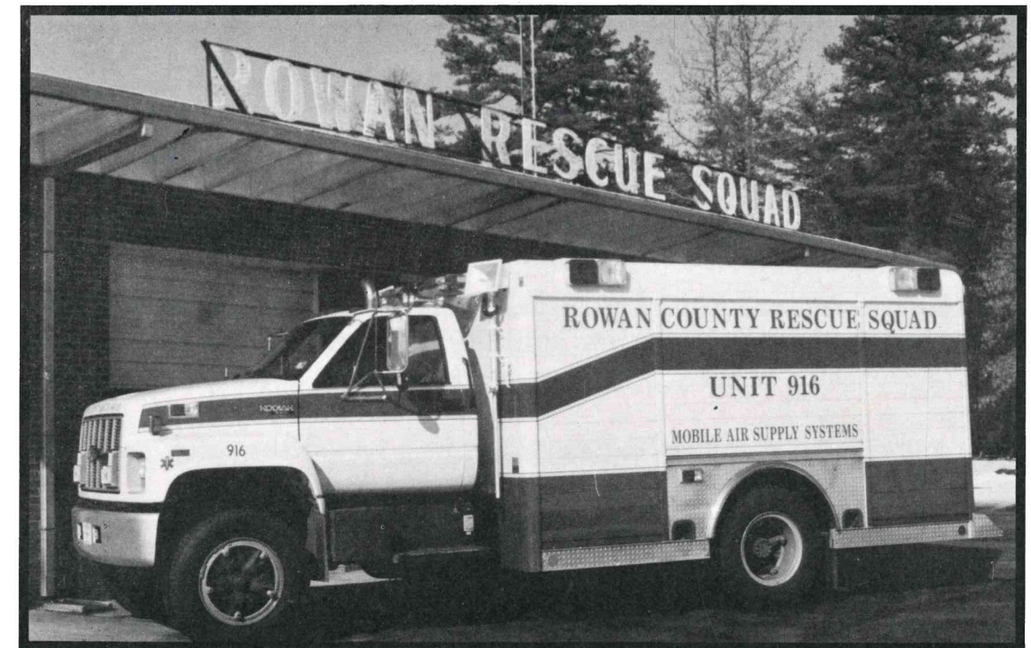
The Mobile Air Supply System was delivered to Rowan County on July 3, 1995. It is mounted on a Kodiak chassis with the body by Hackney and Sons. The compressor, a Bauer K-15, is driven hydraulically. This system was custom built by Safe Air Systems.
