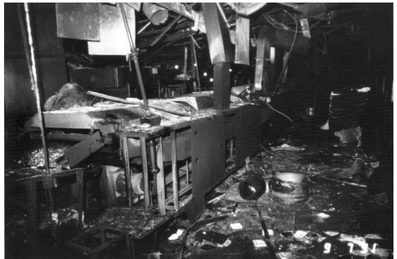
A view of the cooker vat where the fire started.
